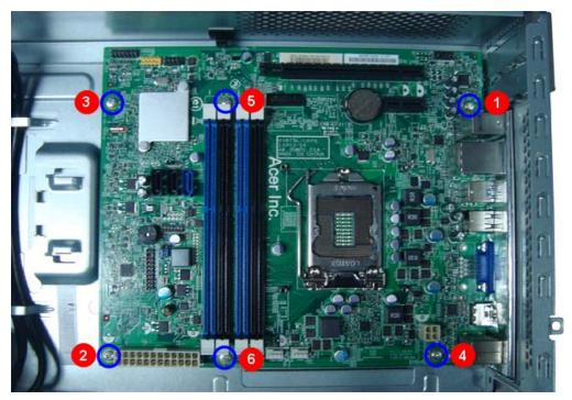
3. Connect the front I/O and optional card reader to the mainboard connectors.
